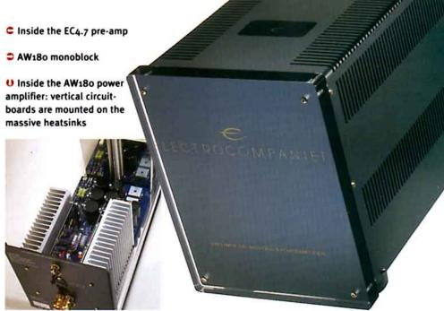
operation with a pair of AW18os per channel. For normal operation (one monoblock per channel) one would either use the non-inverted input, shorting out the inverted one with the dummy plug supplied, or, with a balanced output preamplifier such as the EC4.7, use the XLR input (a looped XLR output socket is fitted, again for bridged operation). The fascia here is formed of 20mm thick acrylic and the company logo is repeated on the top cover, illuminated in red.
